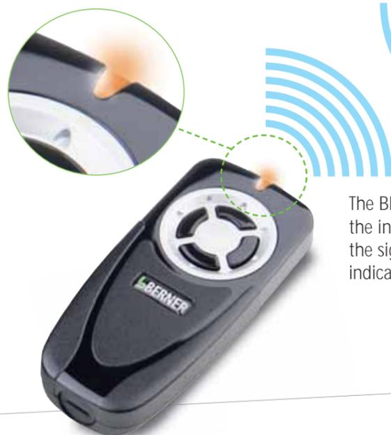
The BDS120 and BDS140 remote controls receive the information from the gate radio receiver that the signal has been transferred securely and indicates this with the orange LED.
